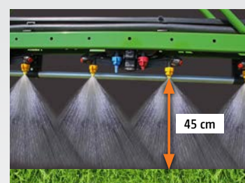
80° nozzles: 25 cm nozzle spacing
