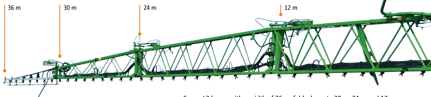
Super-L2 boom with a width of 36 m, folds down to 30 m, 24 m and 12 m
