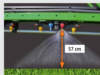
110° nozzles: 50 cm nozzle spacing
