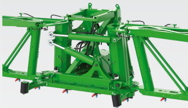
Swing compensation system for L3 booms from 39 metres
