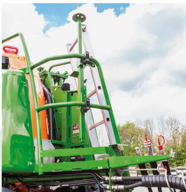
✓ Platform with ladder for easy access to the tank
