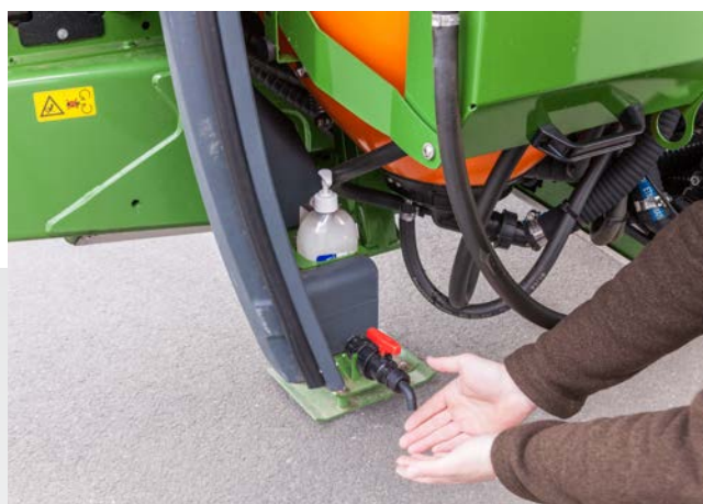
✓ Hand-wash tank with soap dispenser
