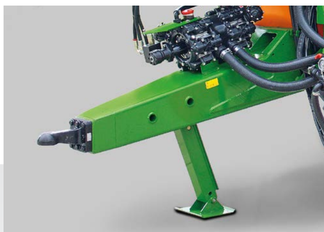
Lower mounted hitch drawbar with K80 ball coupling and hydraulic parking jack
