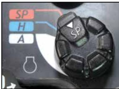
The X3 has three engine work modes to give the operator full control of the machine for the job at hand:
