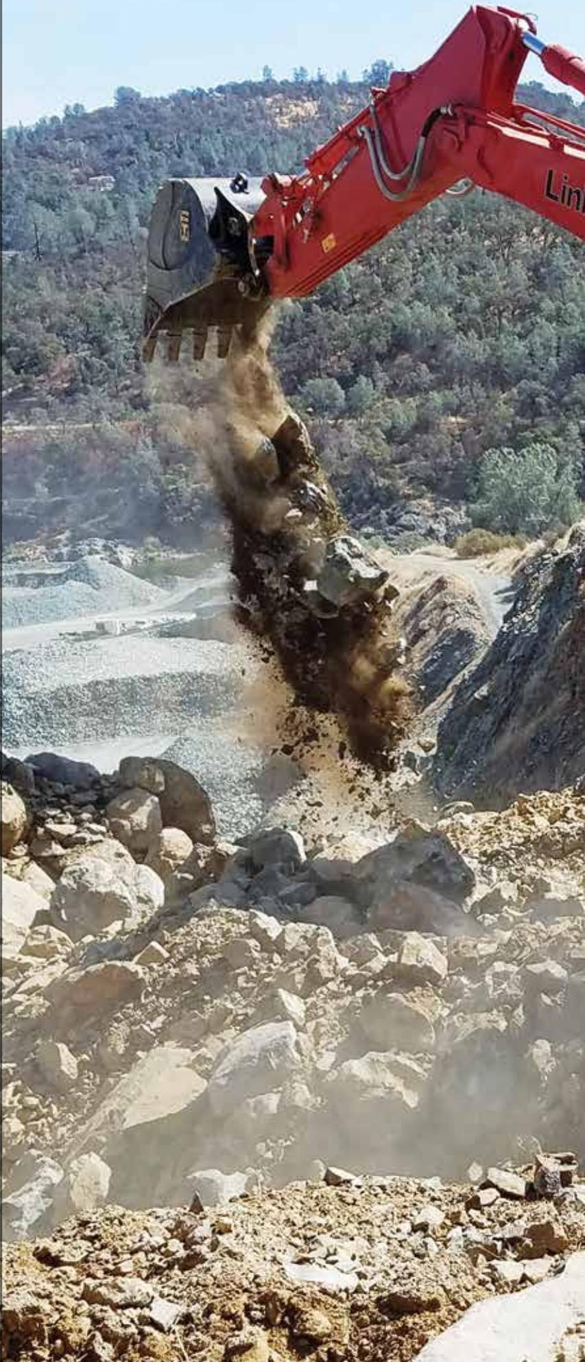
Greater digging power and increased lift capacities are the result of our innovative Spool Stroke Control (SSC) system, which reduces pressure loss and distributes hydraulic oil more smoothly. Pilot pressure sensors detect the type of work being done—such as digging or leveling—and then relays that data to proportional solenoid valves that quickly determine where optimal hydraulic pressures should be directed for that operation.
