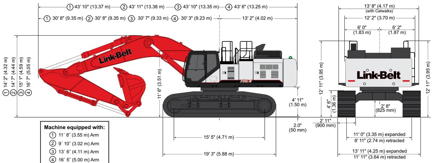
Machine equipped with:
