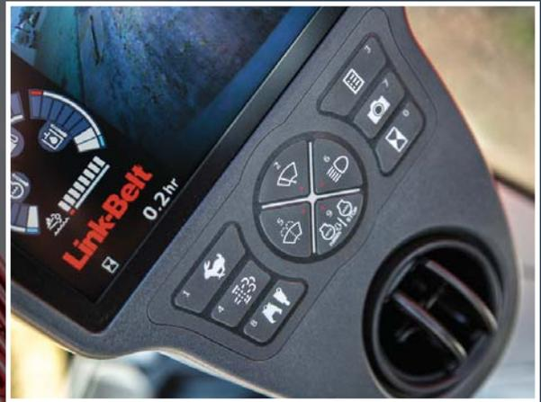
High-Definition LCD monitor has a full-color 7" display that rivals the resolution found in luxury automobiles. Controls are easy to read and easy to use. The rear-view camera activates automatically whenever the machine is started, and sight guidelines have been added for increased safety.
