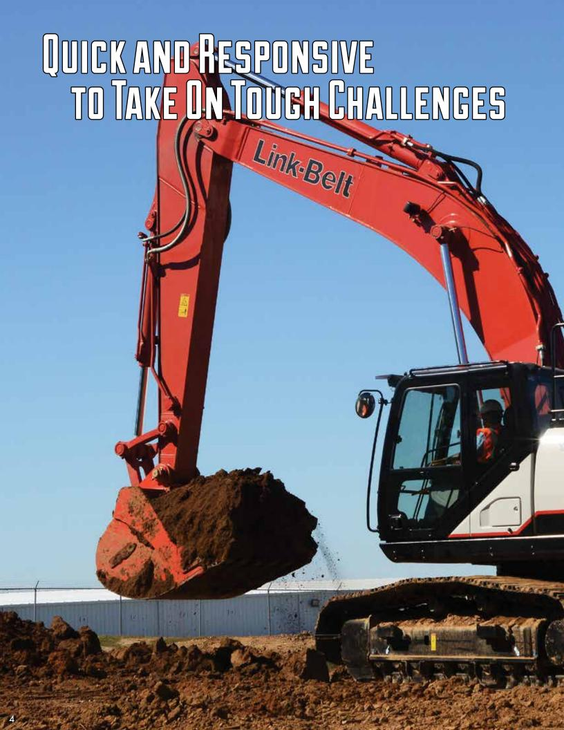
Greater digging power and increased lift capacities are the result of our innovative Spool Stroke Control (SSC) system, which reduces pressure loss and distributes hydraulic oil more smoothly. Pilot pressure sensors detect the type of work being done-such as digging or leveling-and then relays that data to proportional solenoid valves that quickly determine where optimal hydraulic pressures should be directed for that operation.
