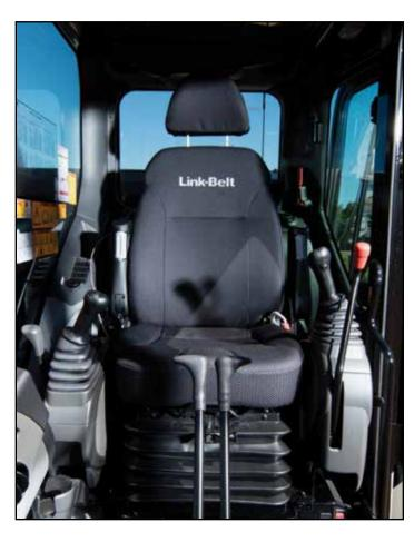
The X4 Series offers the most advanced and roomiest cab in its class. Comfortable, automotive-grade high-back seat with head rest provides superior lumbar back support. With a longer and wider seating surface, it reclines to a 155° maximum reclining angle to create a relaxed environment during breaks. Mechanical suspension is standard, with air suspension, seat tilting adjustment and seat heaters available as options.
