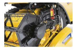
**REGULATE REEL SPEED** Hydraulic reel drive ensures constant reel speed while providing the ability to fine tune reel speed when working in different crops. The result: more efficient harvesting that is gentle on the crop while maintaining productivity.
