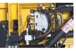
CUSTOMIZED KNIFE SPEED Knife speed ranges from 0 to 630 rpm to ensure that you have the correct cutting speed for all crops. This is adjusted via a valve on the rear of the header.
